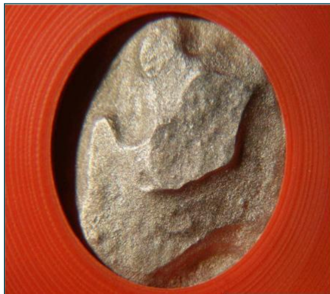
Figure 10 Picture of a.c. coupon on which corrosion had occurred
